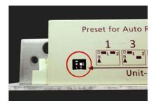
The time delay is selectable by means of a pair of switches accessible at the side of the lock body (FIG 1- 10).
