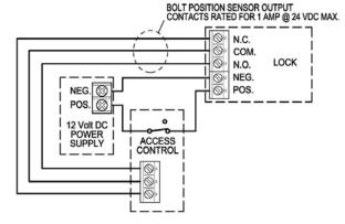
FIG. 4 WIRE CONNECTIONS
