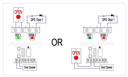
Automatic doors, rollups and motorized sliding doors can be configured as locked doors (the output follows the REX input if no interlocked doors are open) or they can be treated as unlocked doors where the relay breaks the "OPEN" request circuit inhibiting the opener when an interlocked door is open.
