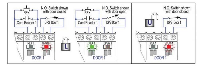
Verify the input light is lit for every interlocked door. Remember, door switch closes when door is closed.
