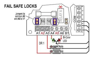
The convention for Dortronics controllers is fail safe - the relay energizes to lock the door. Connect mag locks to the normally open contacts. Connect other lock types for the desired operation.
