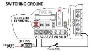
Some installations require that the lock relay switches the lock ground lead. Relay common must be wired to the ground and the WET CONTACT jumper must be removed to prevent a short circuit and possible damage to the board.
