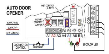
When the relay is energized the door OPEN request circuit is enabled. The LED turns green to indicate that the door may be opened. When the relay is not energized, the door OPEN request circuit is interrupted. The red LED shows that the door is not available for access.
