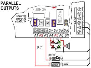
Use Parallel connections to operate multiple devices from a single DPDT relay output. Wet contact jumpers eliminate having to connect relay common head to U4 out tornicate. There is find the device of the device back to V+ out terminals. Though fused for 3 Amps, do not exceed 2 Amp holding current per set of contacts to ensure optimum service life.
