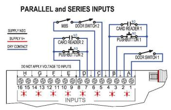
Two or more normally open dry contact switches can be connected in parallel at any input. Similarly, Door Position Switches and Magnetic Bond Sensors (or other sensor outputs) can be connected in series as long as the contacts are dry.
