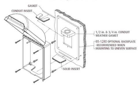
Clear, tamperproof, super-tough polycarbonate shield and frame. Cover is UVstabilized against sun deterioration. Units have standard blue highlight with white lettering
