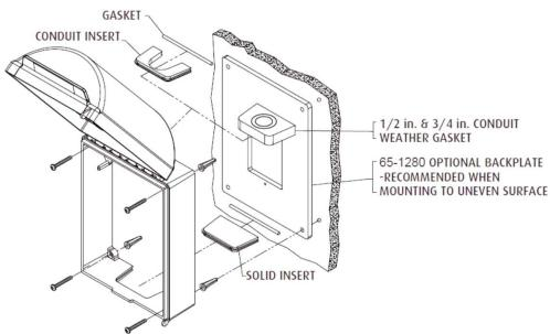
6510/COV/SR (With sounder & Relay) Includes 1 SPDT alarm relay output with contacts rated 1 amp @ 30 VAC/VDC Standard power source is remote 12/24 VDC power source. May also be powered from a 9 VDC alkaline battery (included). Units have standard blue highlight with white lettering
