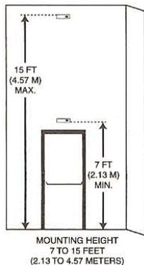
NOTE: If the maximum range of 8.4' is desired, The mounting height must be at the maximum 15' Choose a location that:
