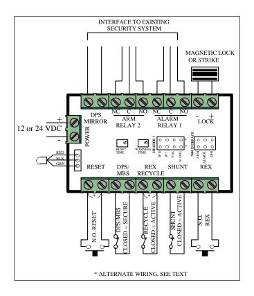
**SETTING THE WARNING TIME:** The warning time is adjustable over the range of 0 seconds to 5 minutes. Referring to the illustration above, use the potentiometer labeled "Warning Time" to adjust the time period. This is a multi-turn adjustment, and is adjustable over a wide time range. The adjustment may be a little tricky if very short warning times are needed. A trial and error procedure will be necessary to get exact times.
