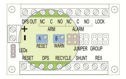
**A - SETTING THE AUTO-RESET TIME:** Use a small screw driver to turn the adjusting screw of the RESET trim pot (A) – clockwise to increase the delay up to 5 minutes and counterclockwise for less or none. This is a multi-turn adjustment. An exact setting or a very short delay may require more than one adjustment.
