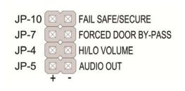
JP5 (AUDIO OUT): Connect a piezo sounder rated for 9 to 12 volts DC to JP5 – observe correct electrical polarity.
